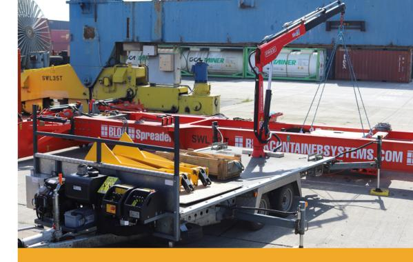
The equipment has had to comply with all the current safety legislation for lifting equipment, plus some additional requirements (as advised by ALLMI) specifically for lorry loader cranes.
